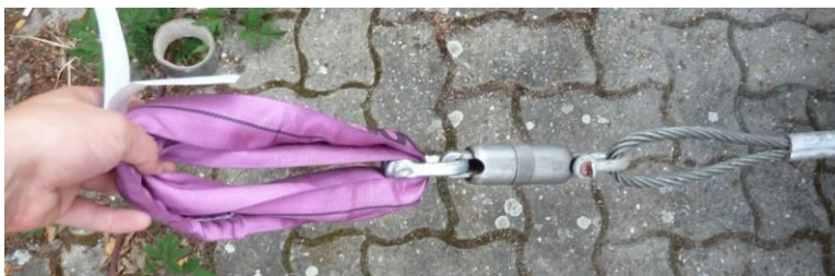
Fig. 3: Incoming groundwater Unsecured shackle
